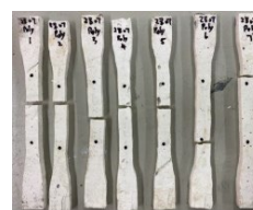
Dog-bone Samples from Tensile Testing
