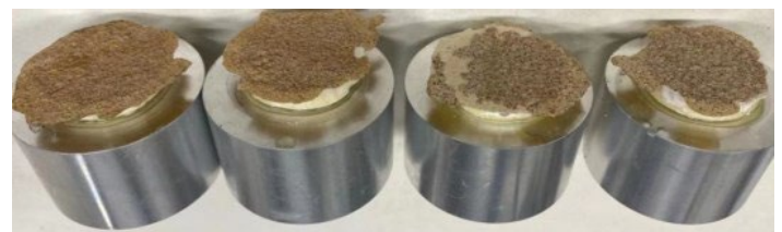
ADHESION TESTING SHOWING SUBSTRATE FAILURE
